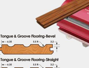
Finishing Planing with Bevel On Two Side End
